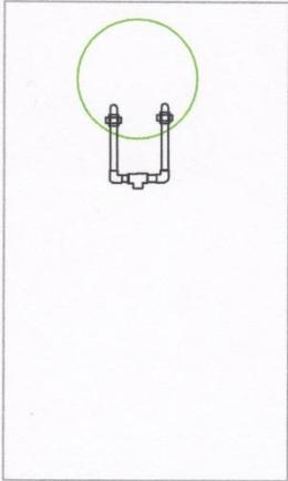
Sewer Popper opening to surface must be at least 6" below sewer line elevation leaving house
